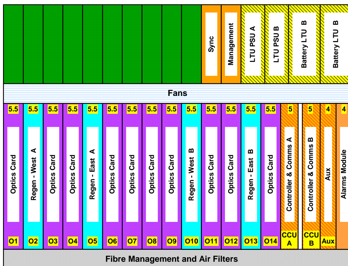
Figure 5: Regenerator Subrack layout
